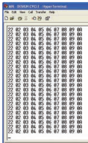
■ SCREENSHOT 2.A 10-byte packet delivered as ordered to the receiver at address 0x22. What you don't see here is the length byte we read and didn't write to the receive buffer, and a CRC at the end of the packet.
