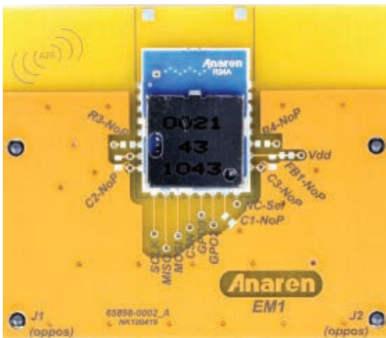
■ PHOTO 3. The A2500R24A-EM1 is the marriage of an A2500R24A AIR module and a Texas Instruments-inspired daughterboard.
