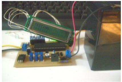
The charger will start to charge the battery, testing it every 30 second (around) and switching to a lower
