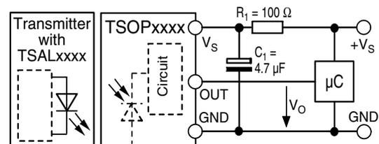
$R_1 + C_1$  recommended to suppress power supply disturbances.
