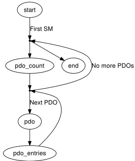
Figure 5.7: Transition Diagram of the PDO Reading State Machine
