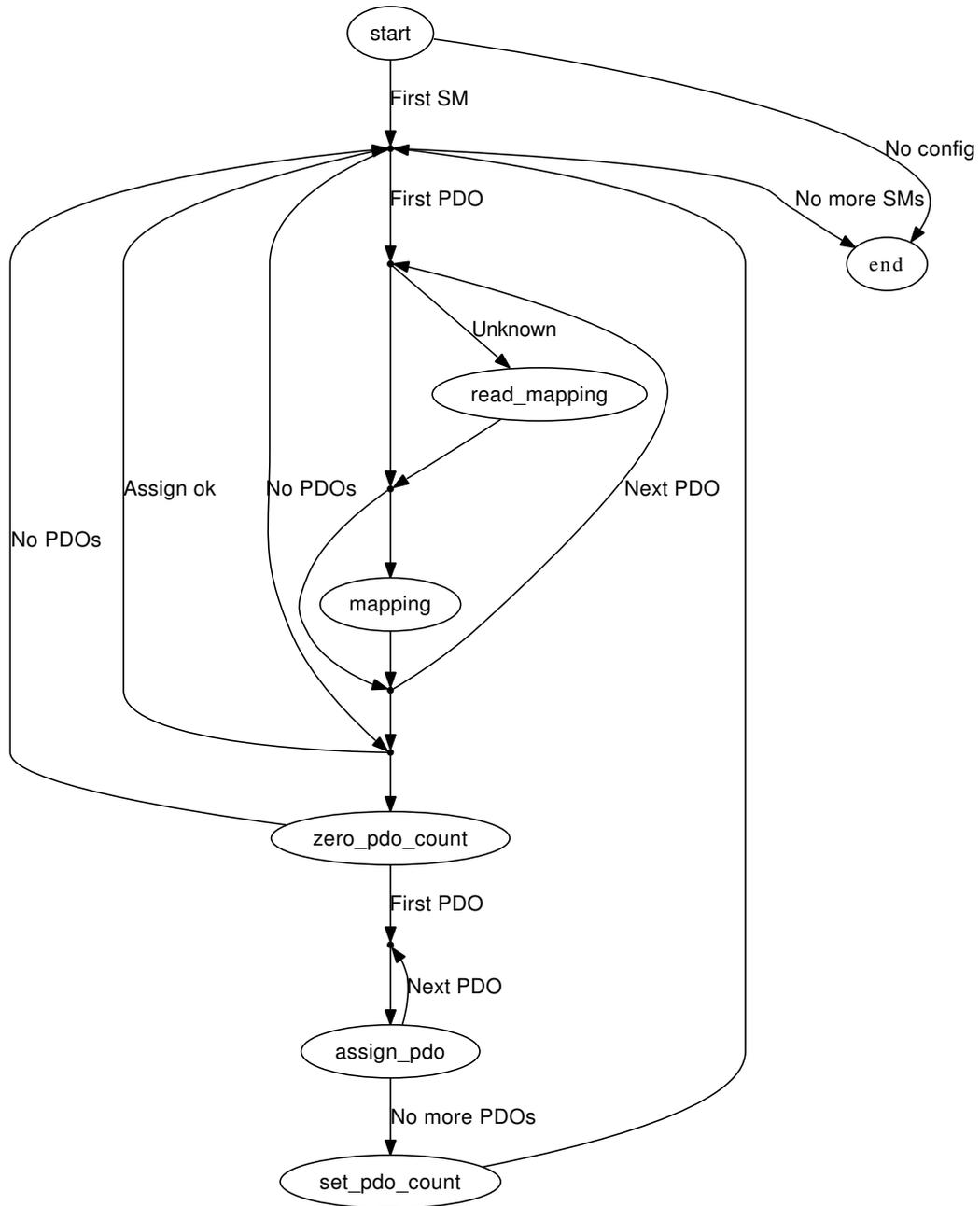
Figure 5.9: Transition Diagram of the PDO Configuration State Machine
