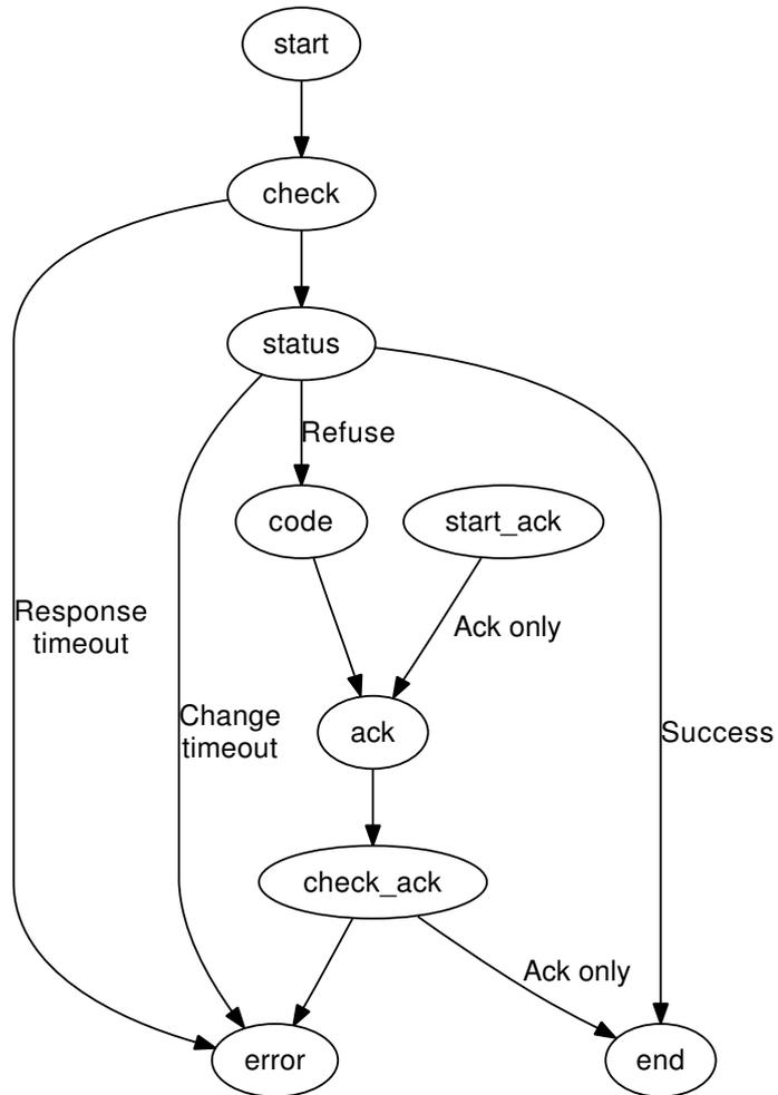
Figure 5.5: Transition Diagram of the State Change State Machine
