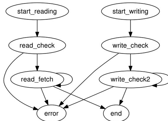
Figure 5.6: Transition Diagram of the SII State Machine
