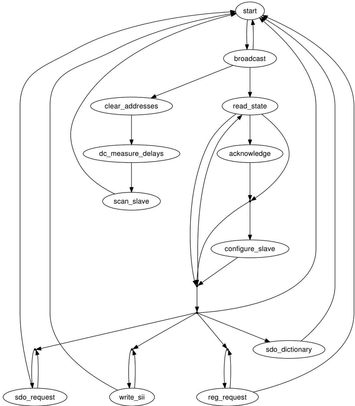
Figure 5.2: Transition diagram of the master state machine
