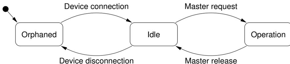
Figure 2.3: Master phases and transitions
