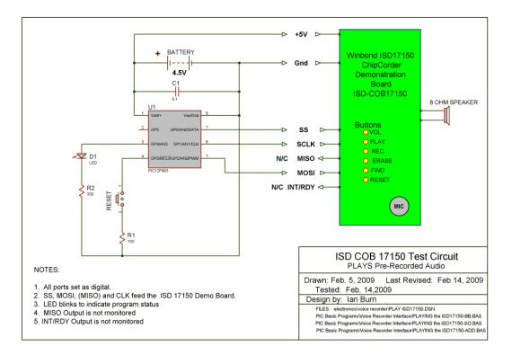
The three output pins on the PIC12F683 that interface with the ISD are GPIO.0 (SS signal), GPIO.1 (SCLK) and GPIO.2 (MOSI). If In-Circuit-Serial-Programming (ICSP) is used with the 12F683, it is necessary to disconnect the Demo Board during programming.
