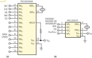
Using the simplified ADPCM algorithm, you can now implement audio capabilities in  $\mu$ Cs by offloading the encoding and decoding tasks onto the parallel (a) or serial (b) mC as if it were a peripheral.
