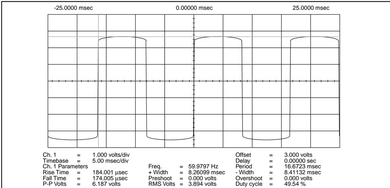
Waveform at part pin (RA0) • R = 100k; Line: 60 Hz, 110V
