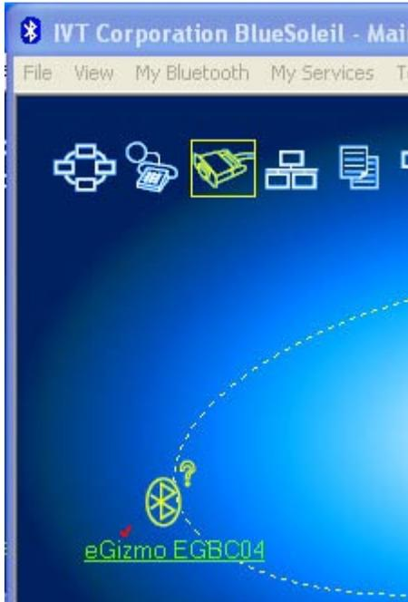
6. Double click on the Serial port Icon top connect with the EGBC-04 serial device. A window will appear similar one shown below indicating the COM port assignment of your EGBC-04 bluetooth service.
