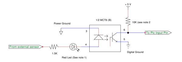
Note 1 : Leds are optional (Useful to monitor sensor state)
