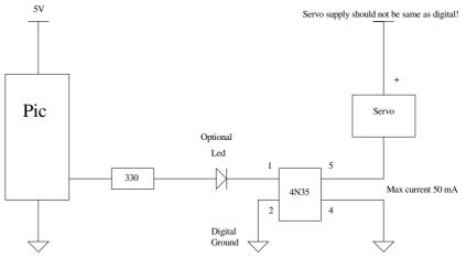
Servo Ground should be separated from digital
