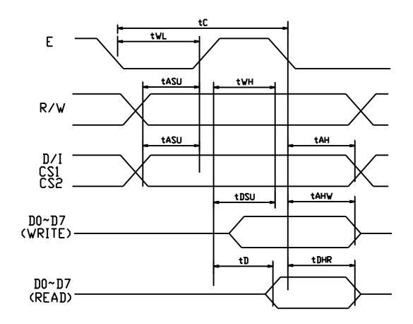
2.Display control timing characteristics (68 type MPU)
