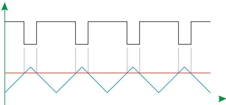
The blue curve represents the triangle wave or counter. The Red line shows the required intensity. When the red line is above the blue curve, the PWM output switches on.
